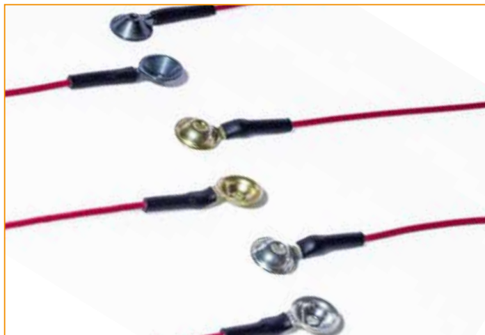
From Top: Ag/AgCl, Au plated, Ag plated
